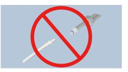
An IEC 3<sup>rd</sup> edition neonate air hose cannot be connected to cuffs with the previous IEC edition snap connector.
